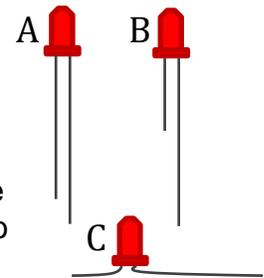
Students will need about 20" of copper tape to complete the circuit. Cut the copper tape in advance of the lesson to expedite circuit construction. They do not need scissors to cut the copper tape. It tears easily with your hands.
